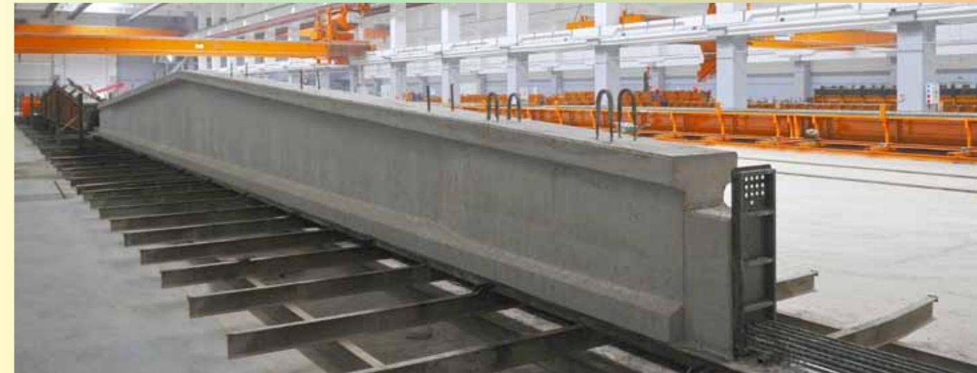
proizvodnja AB montažnih elemenata / production of prefabricated concrete elements
